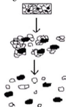
Fig. 8: Schematic representation of Due to disintegrating particle Particles swell to pre compression size and break up matrix
