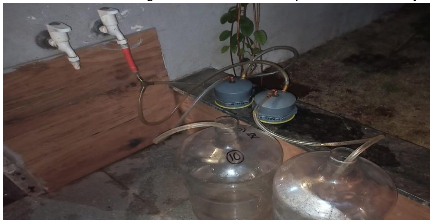
Fig. 1 Household Experimental Setup of PoUCF
